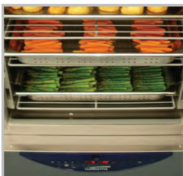
Food is now blast chilled or frozen from +90°C to +3° in 90 minutes
