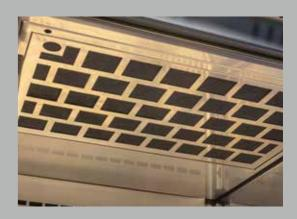
Activated carbon filter removes any organic molecules which cause odur from air circulated within the cabinet.
