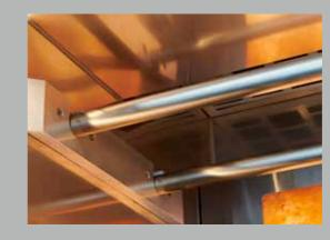
Removable hanging rods support the flexible arrangement in cabinet for the changeable operation flow.
